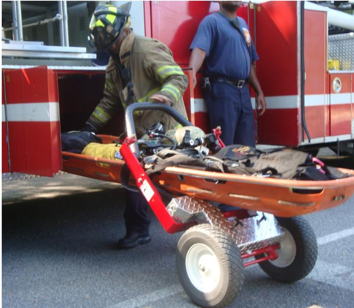
The TURK is a two wheel multipurpose collapsible rescue kart that offers various functions for first responders when dealing with Rescue, Rapid Intervention, Hazardous Material, and Mass Casualty Incidents. Its adaptability to situations where manpower is limited and speed is crucial such as a combat operation is ideal. The TURK can be kept in a folded position stored in a compartment or mounted on the exterior of the apparatus.
